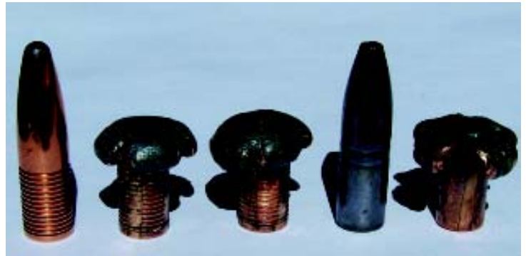
Left to right - Solid shank bullets. North Fork 9.3 mm 286 grain solid shank soft nose before firing, followed by two of the same fired into elephant. Next is a Rhino 9.3 mm 286 grain soft nose before firing, and another fired into an elephant.
