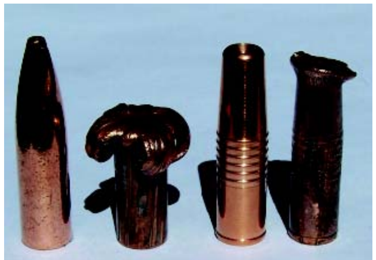
Left to right - Solid copper bullets. Barnes X 9.3 mm 286 grain bullet new and recovered from elephant, followed by North Fork 9.3 mm 286 grain Cup Nose new and recovered from elephant. The North Fork achieves lower pressures, higher velocities, less copper fouling, more penetration and greater accuracy than the Barnes, and the author feels the North Fork Cup Nose is an ideal buffalo bullet.
