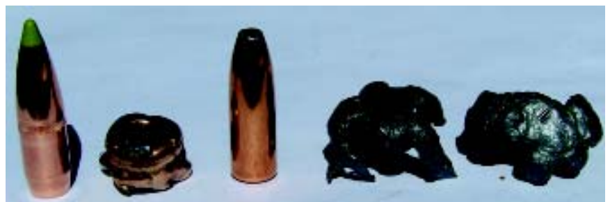
Left to right - Woodleigh 9.3 mm 320 grain soft before firing, followed by the same recovered from an elephant. Next, Woodleigh 9.3 mm 286 grain soft before firing, followed by recovered bullet. The Woodleigh 320 grain soft had far greater penetration than the 286 grain and the author would favour the 320 grain for hunting any game over 400 pounds. Although Woodleigh bullets have the lead core bonded to the jacket, they can still overexpand if pushed too fast or if they hit heavy bone.
