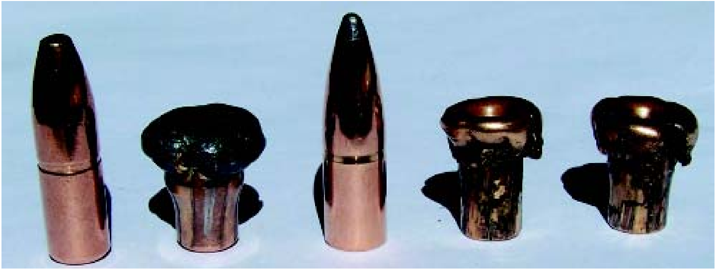
Left to right - Partition-style bullets. Swift 9.3 mm 300 grain A-Frame before and after firing into elephant followed by Nosler 9.3mm 286 grain Partitions before and after firing into elephant. The Swift A-Frame is a far superior bullet to the Nosler Partition whose performance is only mediocre compared to other bullets tested.
