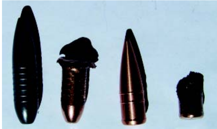
Left to right - Solid copper driving band bullets. GS Custom HV 9.3 mm 265 grain bullet followed by one of the same recovered from elephant. Lutz Moeller 9.3 mm 183 grain Kupperjagdgesschoß bullet followed by the same recovered from elephant. Both bullets were extremely accurate and are excellent for long range. Velocity from the Lutz Moeller bullet is surprisingly high owing to its light weight and minimal contact with the bore.
