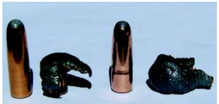
Left to right - Woodleigh 9.3 mm 320 grain soft before firing, followed by the same recovered from an elephant. Next, Woodleigh 9.3 mm 286 grain soft before firing, followed by recovered bullet. The Woodleigh 320 grain soft had far greater penetration than the 286 grain and the author would favour the 320 grain for hunting any game over 400 pounds. Although Woodleigh bullets have the lead core bonded to the jacket, they can still overexpand if pushed too fast or if they hit heavy bone.
